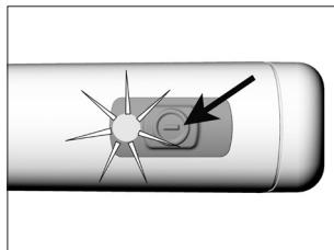
① Press the ON/OFF button on the handpiece drive for 5 seconds.
